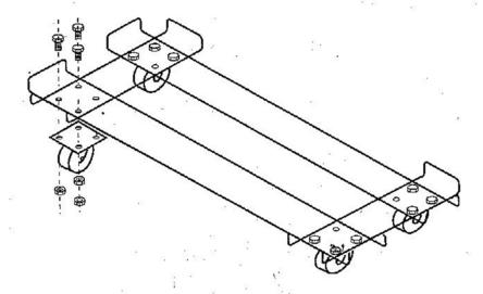
Place Bin firmly on Base and secure down with 2 Straps and remaining Nuts and Bolts.
