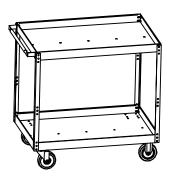
5. Bolt Horizontal Beam (H) to Lower Tray (B). Hardware: 5pcs HW5 and 5pcs HW6
