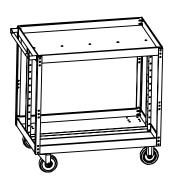
7. Bolt Horizontal Beam (H) to Upper Tray (A) (insert bolt down) and Vertical Rails (G). Hardware: 5pcs HW5 and 5pcs HW6; 4pcs HW1.
