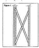
5. Bolt the X-braces to the inside of the posts near the midpoint. Note: Bolt heads should be outside of the frame.
