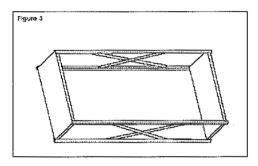
Note: All shelves are bolted from the front and back, thru the short leg of the post. The shelves are not boited thru the long leg of the post thru the side of the shelves. The heads of all bolts should be outside of the unit. All nuts are in the inside of the unit.
