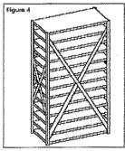
Note: Bolt heads should be outside of the trame
