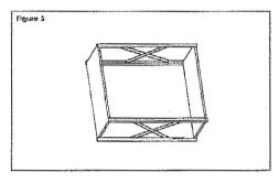
Note: All shelves are boited from the front and back, thru the short leg of the post. The shelves are not bolted thru the long leg of the post thru the side of the shelves. The heads of all bolts should be outside of the unit. All nuts are in the inside of the unit.
