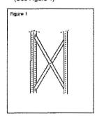
5. Bolt the X-braces to the inside of the posts near the midpoint. Note: Bolt heads should be outside of the frame.
